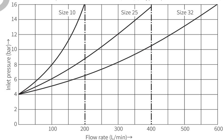
The curves are valid for outlet pressure  $P_B=0$  over the entire flow range.
